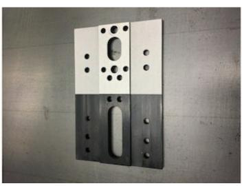
Laser systems remove corrosion, grease, residue and existing coatings from metal surfaces quickly. Source: Laser Photonics
