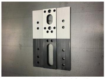
Laser systems remove corrosion, grease, residue and existing coatings from metal surfaces quickly. Source: Laser Photonics
