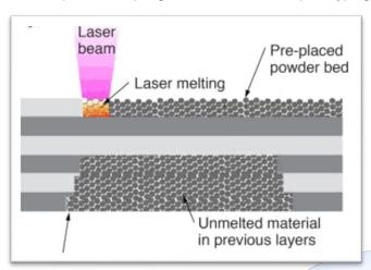
new emerging technically driven applications in high-tech engineering and electronics. 3D Laser Metal Printing is a layered, digitally driven additive manufacturing process that uses high quality focused laser energy to fuse metal NANO powders into 3D objects.
